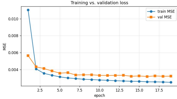
Fig. 3. Training and validation MSE for the baseline (v1). The curves plateau early and track each other with a small gap, indicating a representational ceiling rather than under-training or over-fitting.
